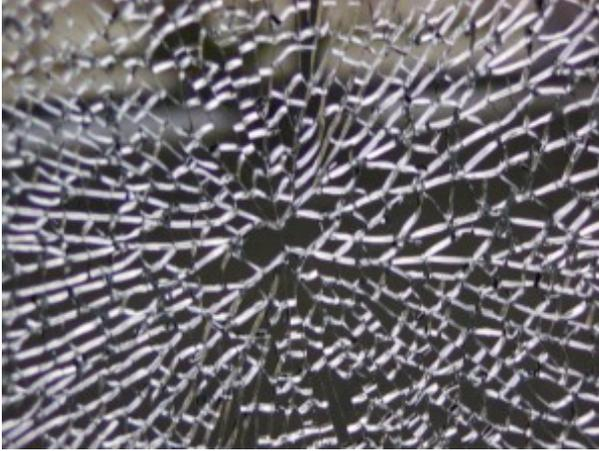
When tempered glass is broken (as shown above), it shatters into thousands of tiny pebbles, practically eliminating the danger of human injury caused by sharp edges and flying shards of glass.
